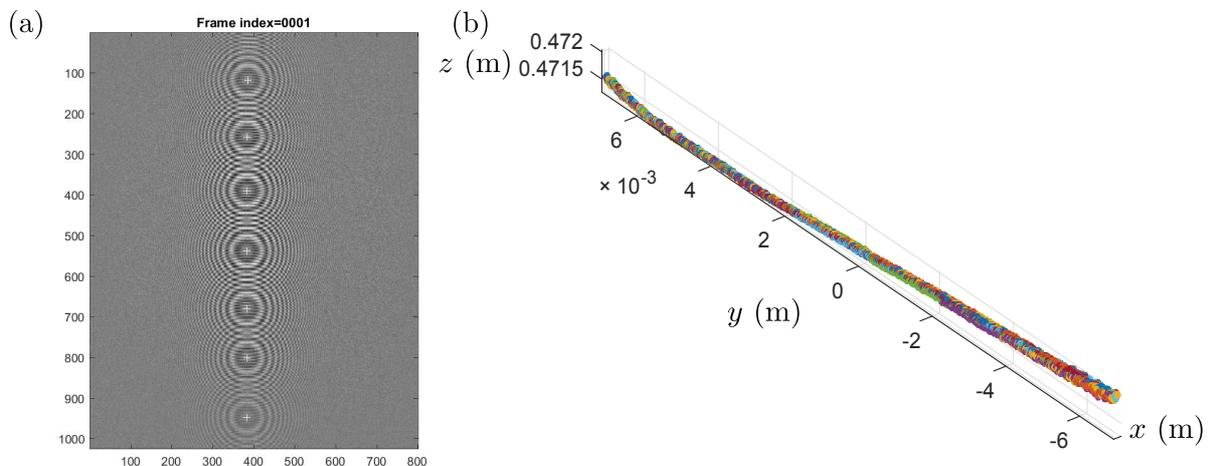
**Figure 5.** (Color online) Example of particle tracking. (a) Parallel tracking of each particle in the hologram (full video sequence is available in Media 1). (b) Extracted 3D-trajectories for all the objects detected.
