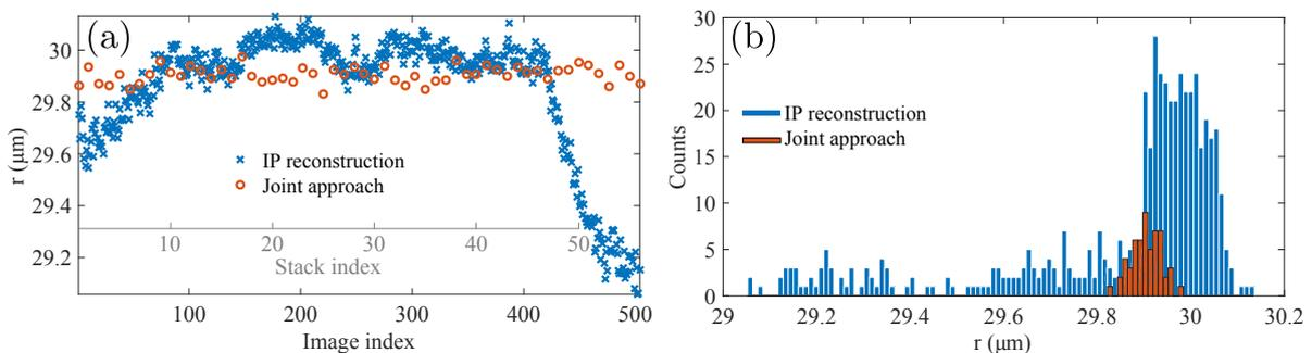
**Figure 6.** (Color online) Evolution of the estimated radius in trajectory 11. Results obtained for classical IP reconstruction are in blue, the joint reconstruction estimates are in orange. (a) Evolution of the radius as a function of the image/stack index. (b) Statistical distribution of the estimated values of the radius (Histogram for all the trajectories are given in Media 2).
