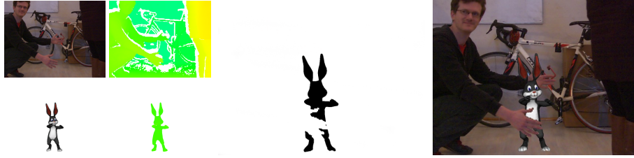
Fig. 4. Example of compositing. Left: first row: film frame and registered depth map, second row: virtual character frame and depth map. Middle: binary mask. Right: final compositing
