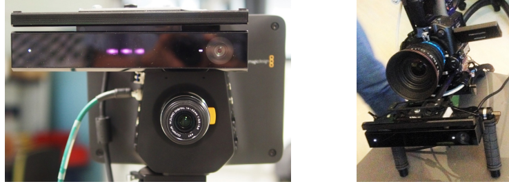
Fig. 3. Our system using different film cameras coupled with the Kinect 2. Left: Blackmagic Studio HD with 14mm lens. Right: Panasonic AG-AF100A with a 18mm lens
