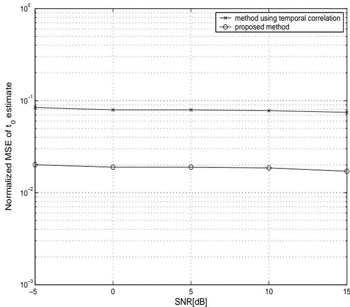
Figure 4: Normalized Mean Square Error of  $\hat{t}_0$ . Case of AWGN channel.
