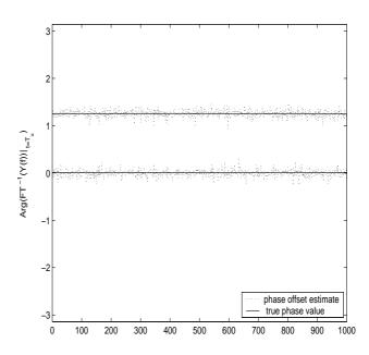
Figure 1:  $\Phi_{f_c}^1$  estimation for  $\Delta f_c = 0$  and  $\Delta f_c = 1/5T_u$ . AWGN channel with SNR = 10dB.
