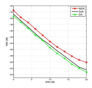
Fig. 5. MSE vs SNR, BPSK signal, normalized time delay=0.1,  $\alpha = 0.5$
