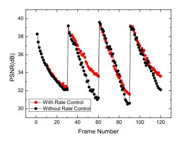
Fig. 5. Performance comparison between using rate control and without rate control (fixed source coding 96Kbps)
