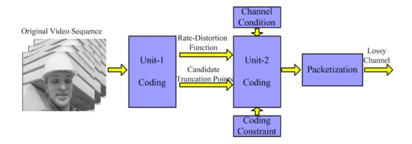
Fig. 1. The architecture of JSCC.
