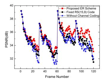
Fig. 6. Performance comparison between the proposed JSCC scheme with the representative fixed channel coding and without channel coding scheme.
