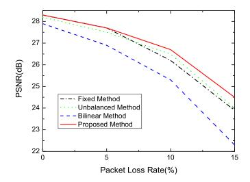
Fig. 7. Performance achieved by proposed method for the Weather forecast sequence, at the  $r_b = 96$ Kbps and  $L_B = 4$ .
