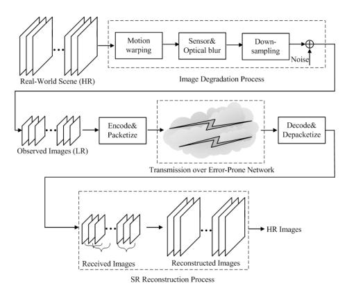
Fig. 1. The total architecture of video transmission and processing
