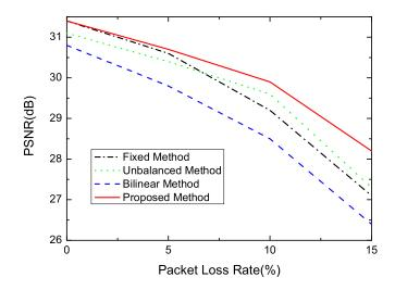
Fig. 8. Performance achieved by proposed method for the Weather forecast sequence, at the  $r_b = 256$ Kbps and  $L_B = 4$ .
