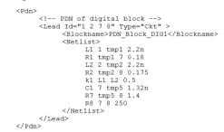
Fig. 2. Example Pdn section defined using a Spice-like netlist
