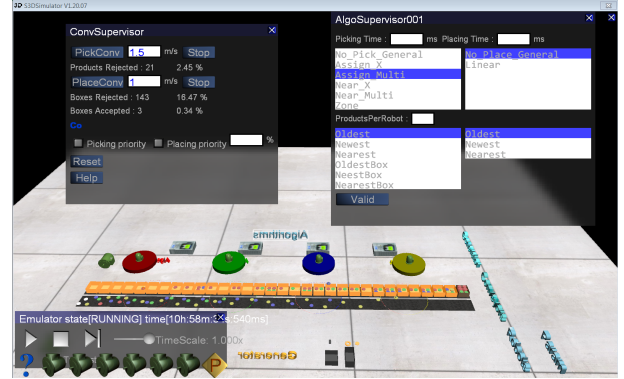
Fig. 4. Simulation example with four robots and two conveyors co-current with the Right/Left collaborative strategy.
