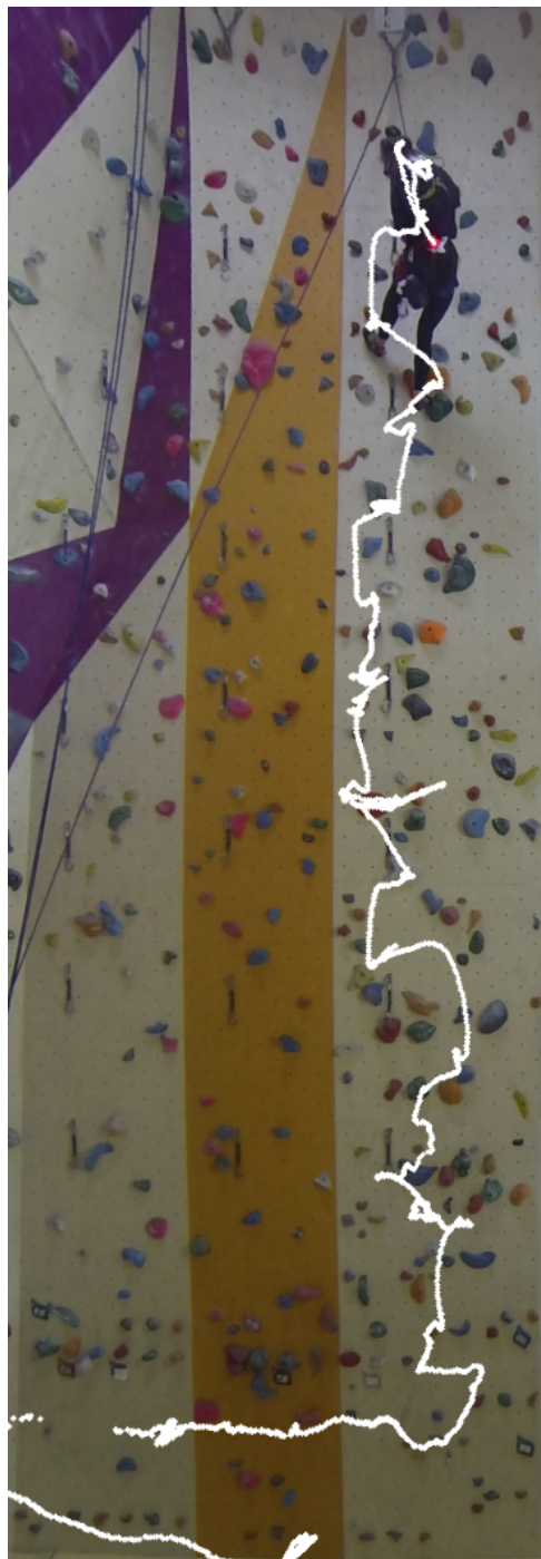
Fig. 3. Example of automatic tracking of the climber based on video footage. The trajectory during the climb is shown in white. The background image is the last image from the video, therefore containing the last tracked position. It is also apparent that the red light can be hidden, for example, due to substantial body rotation so that the light no longer faces the camera. On this image, the lens distortion and the parallax were corrected.
