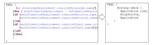
Figure 8: Model-To-Text (FEEL) transformation with Acceleo module
