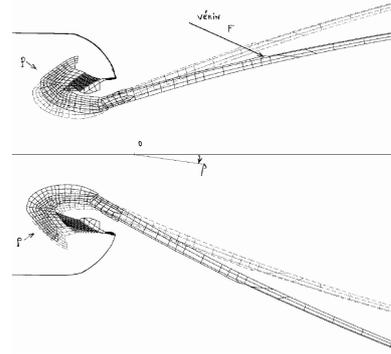
Figure 3: Axial view of reference and deformed structure
