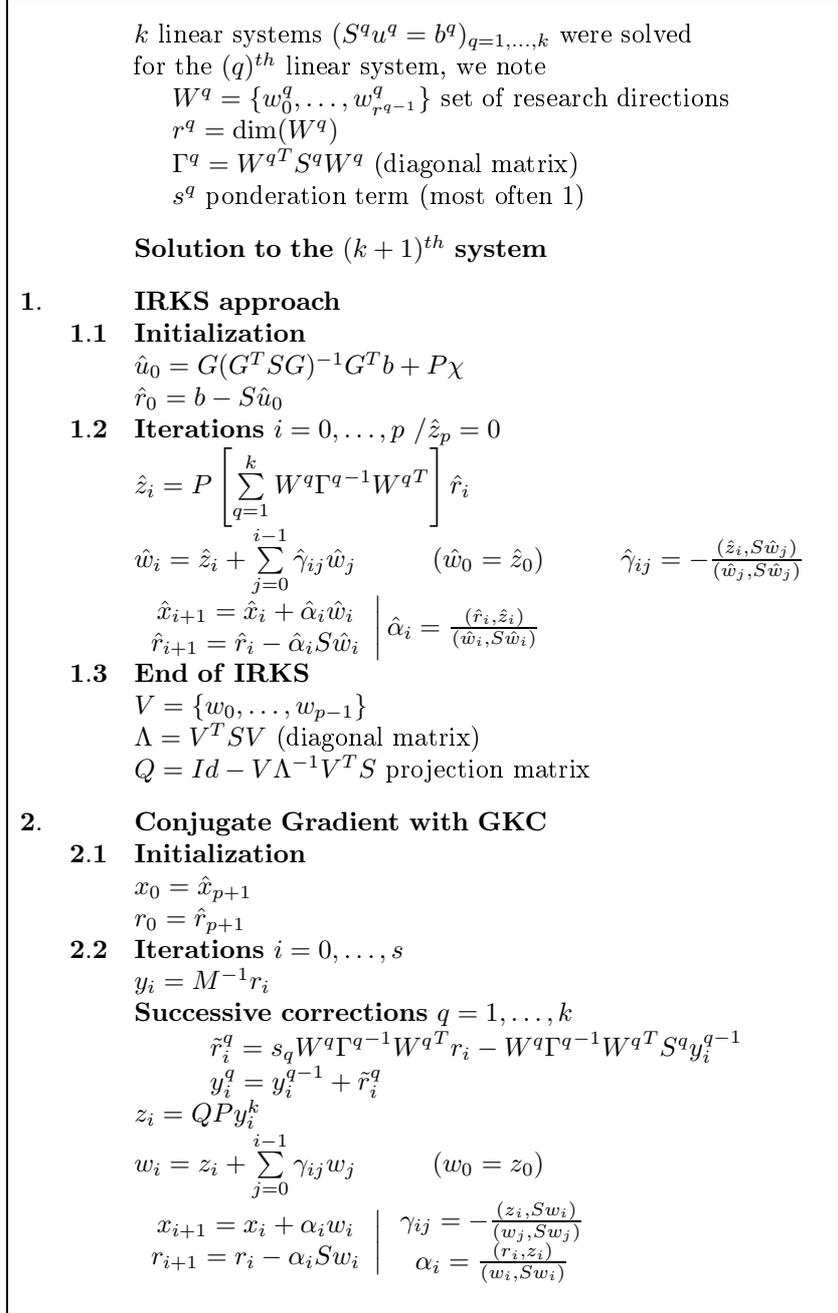
Figure 1: Algorithm: GIRKS with Projected Preconditioned Conjugate Gradient
