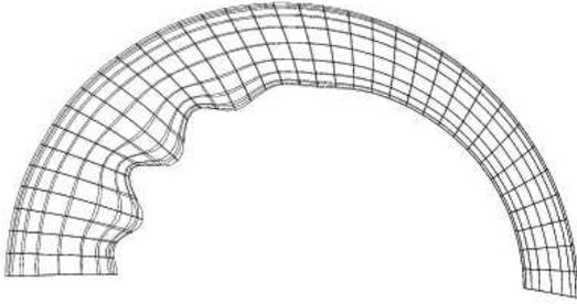
Figure 5: Buckling of one reinforcement
