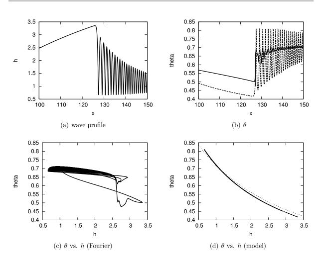
**Figure 6.** Comparisons of the solutions to the FOURIER equation and to the model for a large solitary wave. The solid (dashed) line refers to the FOURIER (model) solution.  $\theta^{(0)}(h) = 1/(1 + B h)$  is compared to  $\theta$  in panel (d) (thin dotted line).
