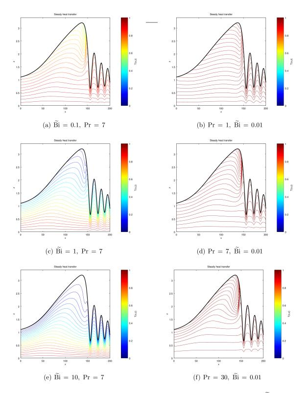
**Figure 2.** On the left column: Isotherms in the inertial frame for different  $\vec{Bi}$  numbers and Pr = 7. As expected, the temperature field is more uniform when no heat transfer is allowed with the free surface. On the right column: Isotherms in the inertial frame for different Pr number. The recirculation zone occurs as the advective part becomes dominant against the diffusive process. Heat flux becomes locally strongly non linear.  $\vec{Bi} = 0.01$ .
