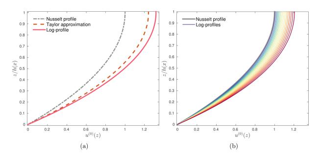
**Figure 3.** Comparison of velocity profiles with  $\Pi_{\mu} \neq 0$ . Physical parameters  $h = 1, A = 0.1, \Pi_{\mu} = 0.25$ . On the right panel (b) the parameter  $\Pi_{\mu}$  changes uniformly from 0.01 to 0.25.
