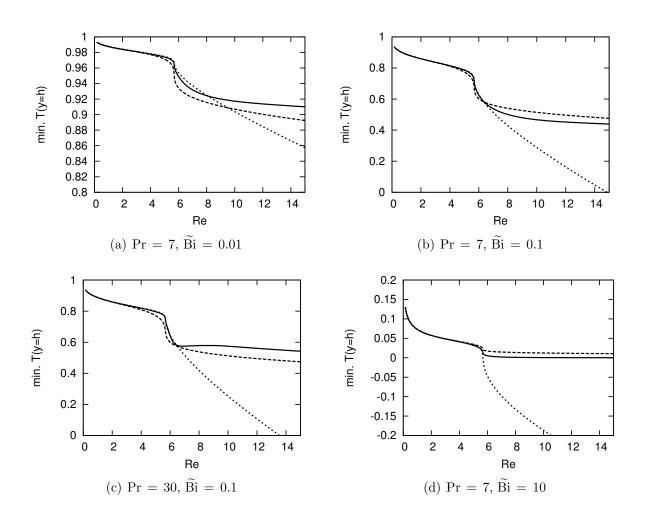
**Figure 5.** Free surface temperature as function of the REYNOLDS number for solitary-wave solutions to the FOURIER equation (solid lines), to system (3.24) (dashed line) and to the averaged energy balance (3.25) (dotted line).
