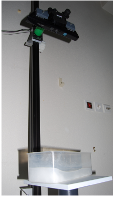
Figure 10. 3D water surface geometry estimated with a Kinect sensor: left, picture of the experimental setting when observing a moving wave in a water tank; right, 3D reconstruction of the wave moving in the tank from Kinect acquisitions at t = 0.15, 0.3, 0.45 and 0.6 seconds. All spatial scales are in millimeters. From Combès et al (2011).
