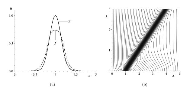
**Figure 2.** Smooth profile propagation under the linear advection equation (2.1): (a) comparison of different profiles (thin solid line is the exact solution, (1) is the numerical solution on the uniform mesh, (2) is the solution on the moving mesh); (b): trajectories of grid nodes in space-time. Note that the panel (a) shows only a zoom of the computational domain.
