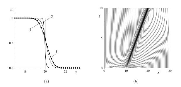
**Figure 1.** Discontinuous profile propagation under the linear advection equation (2.1): (a) comparison of different profiles (thin solid line is the exact solution, (1) is the numerical solution on the uniform mesh, (2) is the solution on the moving mesh and (3) is the first order upwind scheme on the uniform mesh); (b): trajectories of grid nodes in space-time. Note that the panel (a) shows only a zoom of the computational domain.
