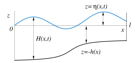
Figure 5. Sketch of the fluid domain in shallow water flows.
