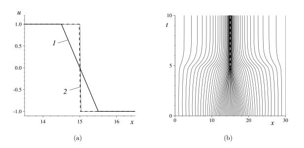
**Figure 3.** Stationary shock wave formation in the BURGERS-HOPF equation: (a) comparison of different profiles (thin solid line is the exact solution, (1) is the numerical solution on the uniform mesh, (2) is the solution on the moving mesh); (b): trajectories of grid nodes in space-time. Note that the panel (a) shows only a zoom of the computational domain.
