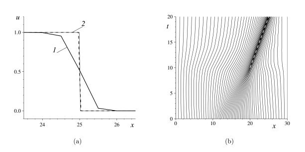
**Figure 4.** Stationary shock wave formation in the BURGERS-HOPF equation: (a) comparison of different profiles (thin solid line is the exact solution, (1) is the numerical solution on the uniform mesh, (2) is the solution on the moving mesh); (b): trajectories of grid nodes in space-time. Note that the panel (a) shows only a zoom of the computational domain.
