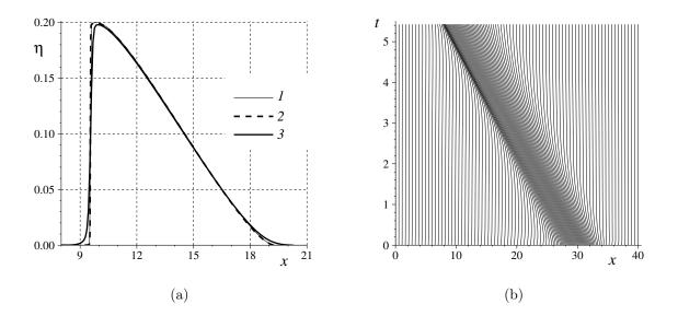
**Figure 6.** Shock wave formation in nonlinear shallow water equations: (a) comparison of different profiles (thin solid line (1) is the exact solution, (2) is the numerical solution on the moving mesh, (3) is the solution on the fixed uniform mesh); (b): trajectories of grid nodes in space-time. Notice that the panel (a) shows only a zoom of the computational domain.
