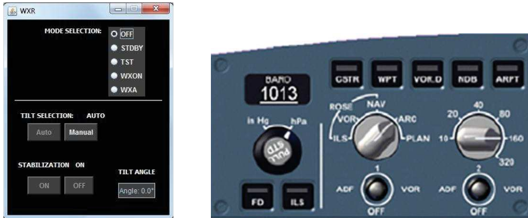
Fig. 1. Image of a) the weather radar control panel b) of the radar display manipulation
