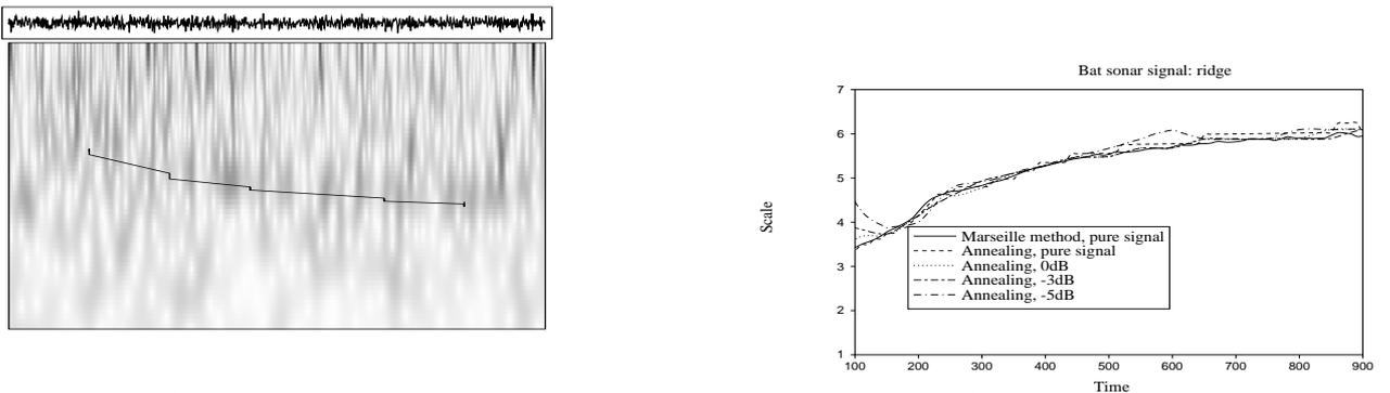
Figure 2: Left) Ridge estimate, snake method;  $SNR = -5dB$ . Right) Comparison of several ridge estimates for the bat sonar signal. Notice that the scale is now increasing upward as opposed to all the other plots where it is increasing downward.
