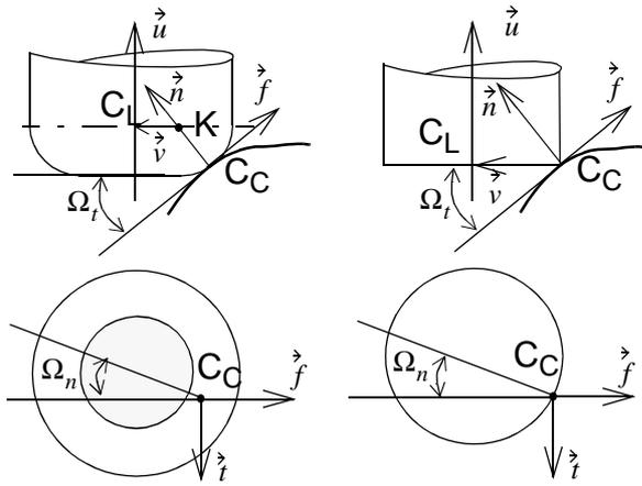
**Figure 6 :** Tool positioning in 5-axis milling
