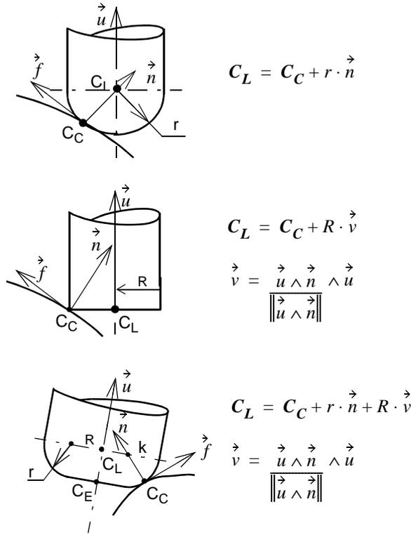
Figure 5 : Tools geometry
