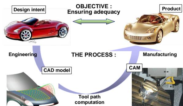
**Figure 1 :** Elaboration process of free-form surfaces
