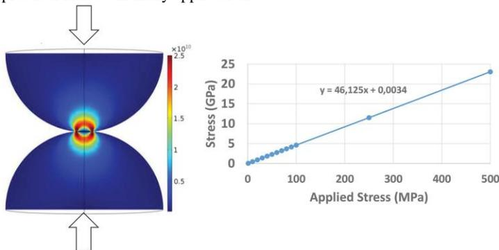
**Figure 7.** Stress at the vicinity of the contact point between two barium titanate half-spheres of 20 nm in diameter as a function of the stress applied on their equatorial surfaces, evaluated by finite element modeling.
