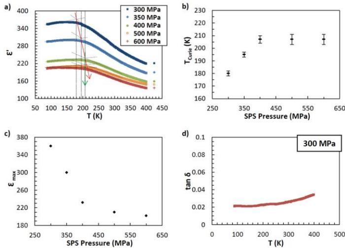
**Figure 5.** a) Permittivity temperature dependence ( $f = 10$  kHz) of ceramics processed at different applied pressures, b) evolution of the Curie temperature as a function of the pressure applied during sintering, c) evolution of the maximum of permittivity as a function of the pressure applied during sintering and d) temperature dependence of the dielectric losses for the ceramic sintered under 300 MPa.
