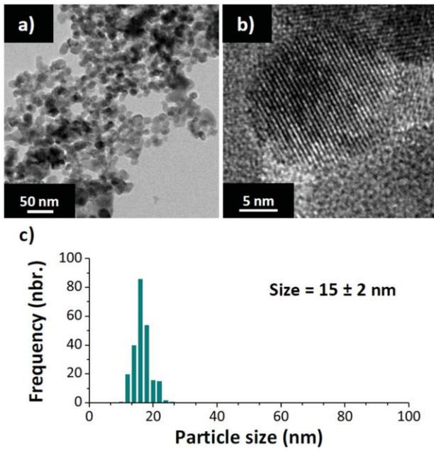
**Figure 1.** a) Transmission electron microscopy (TEM) image of  $\text{Ba}_{0.6}\text{Sr}_{0.4}\text{TiO}_3$  nanoparticles synthesized by supercritical fluids and b) high resolution transmission electron microscopy (HRTEM) image showing the high crystallinity of the particles. c) Crystal size distribution.
