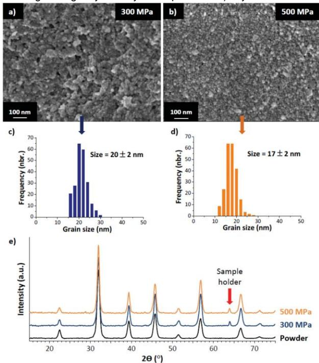
**Figure 2.** a,b) HRSEM images of the fracture surface of the BST ceramics processed by spark plasma sintering at 750 °C under uniaxial pressure of 300 and 500 MPa, respectively; c,d) the corresponding grain size distributions; and e) X-ray diffraction patterns of BST nanopowder and BST ceramics sintered under uniaxial pressures of 300 and 500 MPa.
