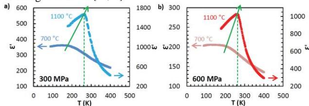
**Figure 6.** Permittivity temperature dependences ( $f = 10$  kHz) of ceramics processed by SPS at a) 300 MPa and b) 600 MPa and annealed at 700 and 1100 °C in each case. Arrows indicate the increase of the Curie temperature after annealing at high temperature.
