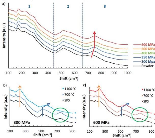
**Figure 4.** Raman spectra of a) BST nanopowder and SPS ceramics processed at different pressures from 300 up to 600 MPa and b,c) ceramics processed by SPS at 300 and 600 MPa, respectively, and annealed at 700 and 1100 °C in each case. Arrows indicate the shift observed in different modes of the spectra.
