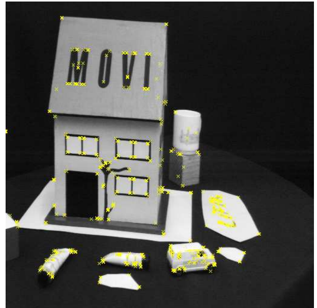
Figure 3: The resulting dominant points detection image on “MOVI” test image.
