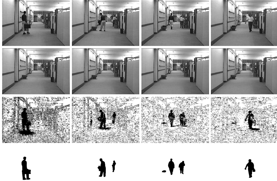
Fig. 3. Background subtraction shown at different frames of the Hall image sequence. Row 1: Original sequence, frames 38, 90, 170 and 250. Rows 2 and 3: \Sigma - \Delta Background and foreground, with N=2 , and T_V = 8 . Row 4: (Fore)ground truth.
