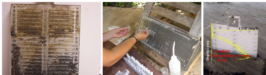
Figure 4. (left) Removal of the dialyser after 20 days equilibration in the sediment, (centre) Porewater sampling using syringes, probes are stored in acidified tubes, (right) ions concentration gradient determination over the depth. Photographs made by V. Mesnage.
