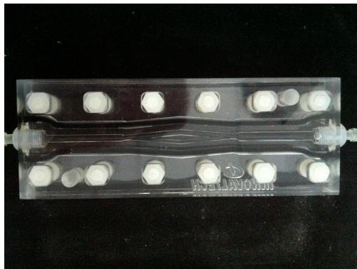
Figure : Physical phantom for cerebral arteries.
