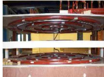
Fig. 2. Induction heating device coils
