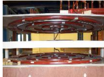
Fig. 2. Induction heating device coils
