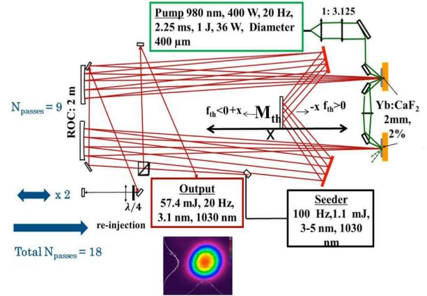
Fig. 8. Experimental setup of the re-imaging multipass amplifier with two Yb:CaF<sub>2</sub> active-mirrors.
