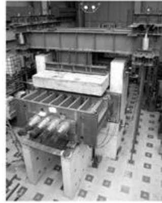
Figure 1. Description of the experiment on the Representative Structural Volume (from (Hermann et al, 2009))
