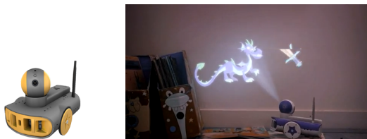
Fig. 1: EMOX, the augmented robot (left). EMOX, projecting a cartoon movie on the wall (right).
