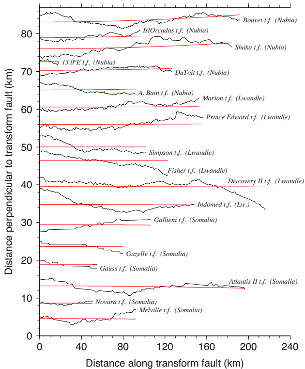
Figure 11. Summary of observed (black) and predicted (red) transform fault traces from Figs 10, 15 and 18, and Supporting Information Fig. S2. Red lines are small circle traces predicted by the C1n rotation poles for the Antarctic plate relative to the Somalia, Lwandle and Nubia plates. Horizontal and vertical axes respectively show the linear distance along each transform fault measured from its southern end and the linear distance orthogonal to each transform fault. The distances displayed on the vertical axis are exaggerated by a factor of four relative to distances shown on the horizontal axis in order to emphasize the misfits and noise in the digitized fault representations.
