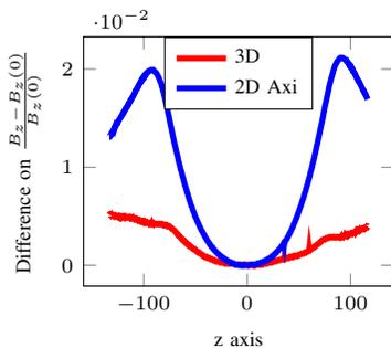
Fig. 3. Comparison of the profile of  $B$  vs the experimental data along  $z$  axis obtained by 2D axi  $B$  (from optimization step) and 3D Biot-Savart calculations
