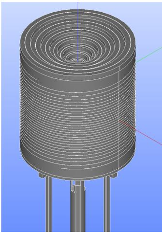
Fig. 1. A 14 Helices resistive insert with current leads
