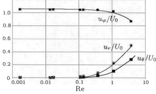
Fig. 5. Evolutions of various velocity field components vs. the Reynolds number Re. The axial magnetic field case. The temperature gradient is  $G_\infty = 3000 \text{ K/m}$ . The magnetic field amplitude is  $B = 0.08 \text{ T}$ . The velocities are normalized by the reference velocity  $U_0$ .
