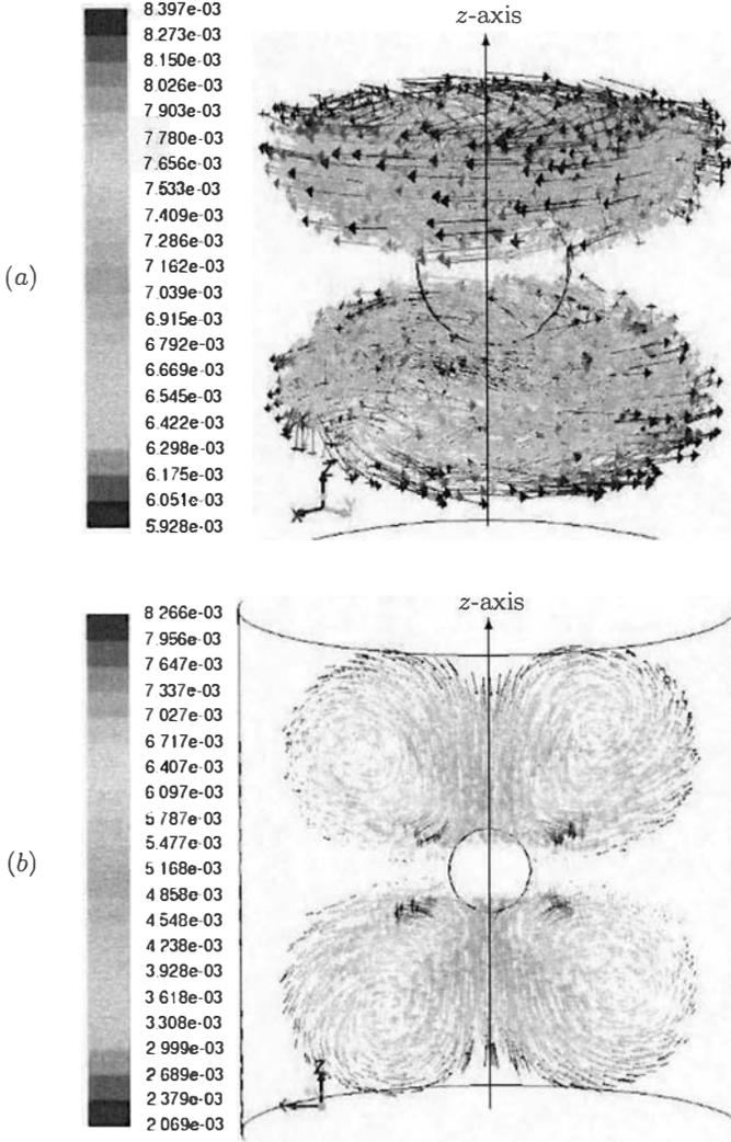
*Fig. 4.* View of the flow pattern around a spherical particle in the case of the axial magnetic field. The parameter values are  $G_\infty = 3000$  K/m, sphere radius  $R = 0.15$  mm,  $B = 0.08$  T. The velocity scale is in m/s. (a) General view of the velocity pattern,  $U_{\max} = 0.0084$  mm/s. (b) View of the secondary flows in the meridian plane.  $Re = 3.67$ .
