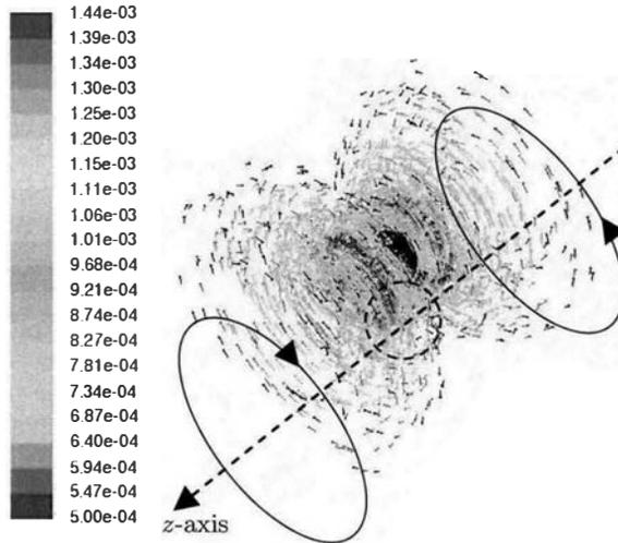
Fig. 3. View of the flow pattern around a spherical particle in the case of the axial magnetic field. The parameter values are  $G_\infty = 3000 \text{ K/m}$ , sphere radius  $R = 0.05 \text{ mm}$ ,  $B = 0.08 \text{ T}$ . The velocity scale is in m/s. General view of two counter-rotating axial vortices,  $U_{\max} = 1.436 \text{ mm/s}$ .  $Re = 0.137$ .
