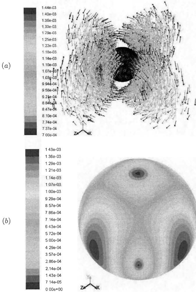
*Fig. 6.* TEM flow generated by a transverse magnetic field. The parameter values are  $G_\infty = 3000$  K/m, sphere radius  $R = 0.050$  mm,  $B = 0.08$  T. The velocity scale is expressed in m/s. (a) View of the velocity vectors. (b) Distribution of the velocity amplitude on a sphere surrounding the particle, the radius of which is close to the maximum of the velocity profile, i.e.,  $2R$ .
