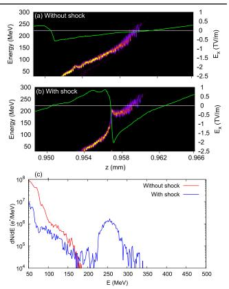
FIG. 3 (color online). Electron density in the phase space (z, E) for a gas jet without (a) and with (b) the shock. The green curve shows the longitudinal electric field on the laser axis. Simulated spectra obtained at the exit are shown in (c). The density transition is at z=0.900 mm.
