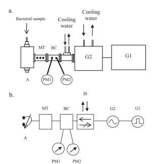
FIG 1 Schematic principles of the experimental DW exposure system. (a) Scheme of the experimental device. (b) Main components: function generator (G1), 2.45-GHz microwave generator (G2), isolator (IS), bidirectional coupler (BC), power meters (PM), and applicator (A).
