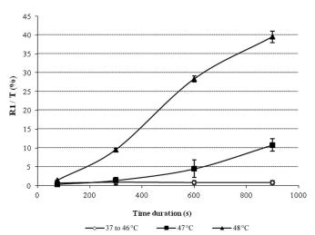
FIG 6 Effect of conventional heating at different temperatures on membrane permeability. Results are expressed as the evolution of R1/T = f(t) for different T (°C) values (where t is time). The curve named "37 to 46°C" corresponds to the average value of the results obtained at 37, 40, 42, 45, and 46°C, since percentages of highly stained cells were similar.
