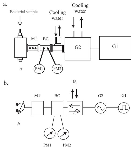
**FIG 1** Schematic principles of the experimental DW exposure system. (a) Scheme of the experimental device. (b) Main components: function generator (G1), 2.45-GHz microwave generator (G2), isolator (IS), bidirectional coupler (BC), power meters (PM), and applicator (A).
