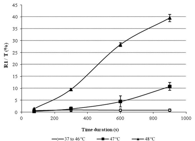
FIG 6 Effect of conventional heating at different temperatures on membrane permeability. Results are expressed as the evolution of  $R1/T = f(t)$  for different  $T$  ( $^\circ\text{C}$ ) values (where  $t$  is time). The curve named “37 to  $46^\circ\text{C}$ ” corresponds to the average value of the results obtained at 37, 40, 42, 45, and  $46^\circ\text{C}$ , since percentages of highly stained cells were similar.
