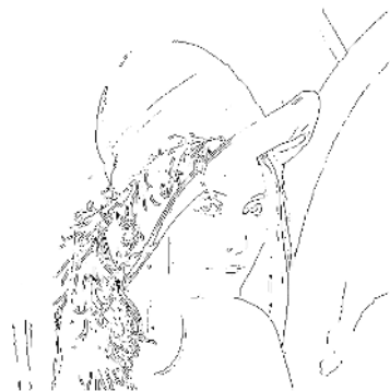
Figure 7. Sobel's edge detector on Lena's gray image.
