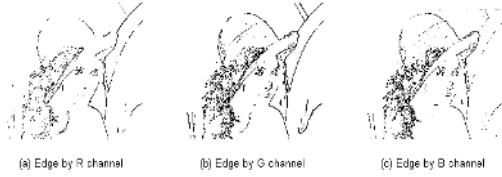
Figure 5. Edge detections in each channel.
