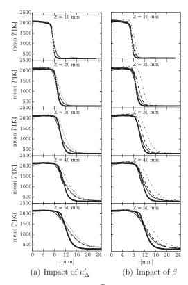
Fig. 7. Mean temperature  $\widetilde{T}$  radial profiles for the stratified case (SwB5) case. Left plot: — 5-NAD-CH1; · · · 5-NAD-CH2; - - - 5-NAD-CO; • • Experiments. Right plot: - · - 5-NAD-B5; - - - 5-NAD-B3; - - - 5-NAD-BD; • • experiments.
