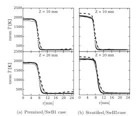
Fig. 4. Mean temperature  $\widetilde{T}$  radial profiles. Legend: ---adiabatic computations (1-AD-CH1 and 5-AD-CH1); — non-adiabatic computations (1-NAD-CH1 and 5-NAD-CH1); •• experiments.
