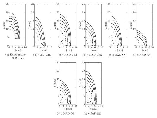
Fig. 8. Cross section in the medium plane of the iso-surfaces of mean axial velocity  $\widetilde{U}_z$  for the stratified case (SwB5). For each figure, isolines values are, from right to left,  $\widetilde{U}_z = \{3; 2; 1; 0; -1; -2; -3\}$  m.s<sup>-1</sup>. Dashed lines:  $\widetilde{U}_z < 0$ ; solid lines:  $\widetilde{U}_z > 0$ .
