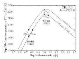
Fig. 6. Equilibrium temperature function of fresh gas equivalence ratio  $\phi$  for adiabatic and non-adiabatic situations. CH<sub>4</sub>-Air fresh gas temperature is taken equal to  $T_0 = 298.0$  K. Legend: upper curve: adiabatic  $(\Delta h = 0)$ ; lower curve: non-adiabatic  $(\Delta h = 1.5 \cdot 10^5)$  J/kg).
