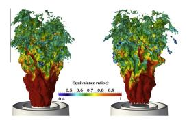
Fig. 3. Isosurface of filtered progress variable reaction rate  $\bar{\rho} \widetilde{\omega}_{Y_c}$  colored by fresh gas equivalence ratio  $\phi$  for the stratified (SwB5) case. Left: Adiabatic computation (5-AD-CH1). Right: non-adiabatic computation (5-NAD-CH1).
