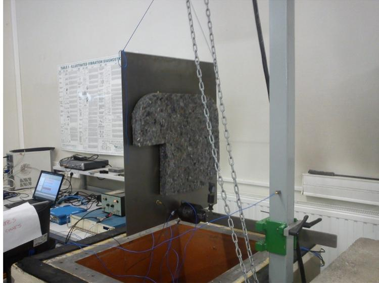
Figure 3: Steel plate excited with a shaker.
