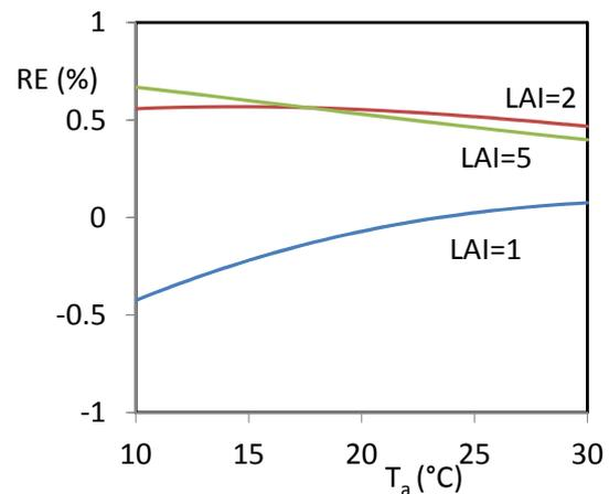
**Figure 3.** For different LAI, RE on crop evapotranspiration  $ET_c$  when it is calculated with the modified Penman–Monteith equation (Eq. 10) compared to the two-layer model used as a reference:  $z_h = 1.5$  m,  $r_{s,s} = r_{s,l} = 100$  m s $^{-1}$ , under sub-humid conditions with  $u_a = 2$  m s $^{-1}$  and  $R_a = 40$  MJ m $^{-2}$  d $^{-1}$ .
