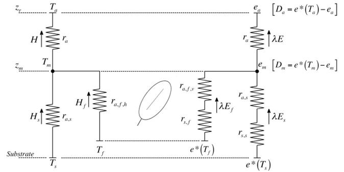
**Figure 1.** Resistance networks and potentials for a two-layer representation of the convective fluxes (sensible heat and latent heat) within the canopy. The nomenclature used is given in the list of symbols.
