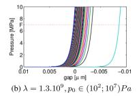
Figure 8: Exponential contact law evolution as function of its parameters
