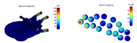
Figure 11: Steady sliding state absolute displacement of a TGV brake using Signorini contact implementation, contact resultant at nodes of the disc top side
