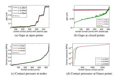
Figure 12: Comparative gaps and contact pressures between Signorini and exponential laws resuls.
