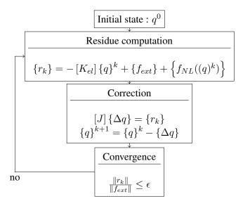
Figure 4: Implementation of a static Newton resolution scheme
