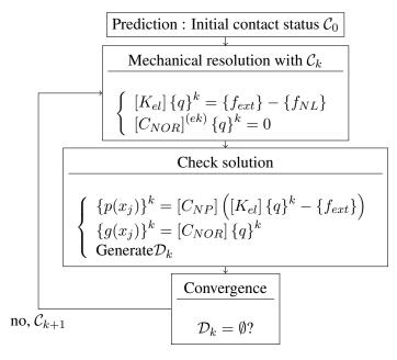
Figure 5: Implementation of an Uzawa resolution algorithm for the sliding Signorini-Coulomb problem using status
