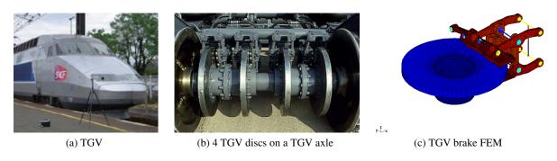
Figure 10: The TGV brake system
