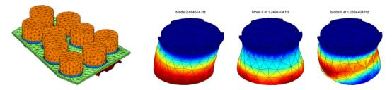
Figure 6: Left: A sample railway braking pad. The friction blocks in orange are linked to the backplate in green, using rings in blue. A dovetail joint (in red) fixes the pad in the brake rig. Right: Sample block modes in clamped/sliding conditions with ideal contact for a ring fitted block
