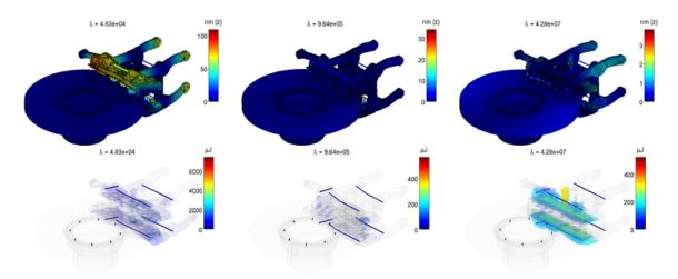
Figure 13: Absolute displacement differences in nanometers between Signorini and functional static results, from top to bottom along the x, y and z axis, from left to right in increasing  $\lambda$ . Strain energy densities of differential displacements are presented for elements with highest levels only
