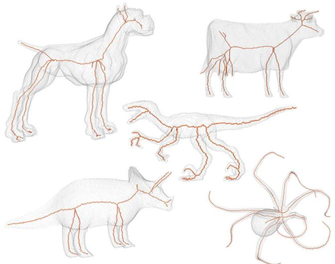
Fig. 10. Curve skeletons computed by `AsymThinningScheme`.
