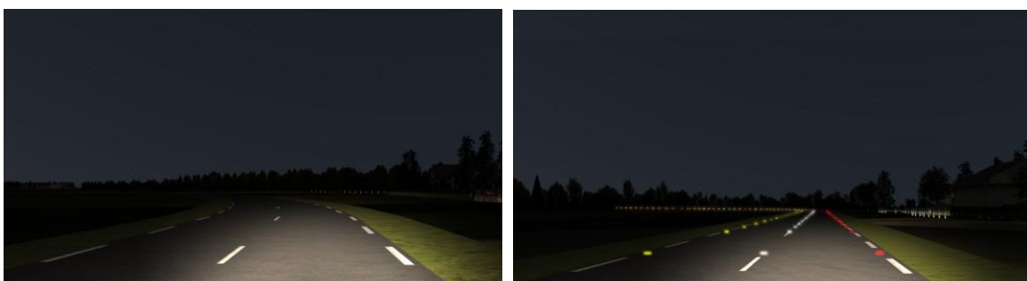
Figure 2. Stud sections for the 150 metres (left) and 400 metres (right) long curves. In both curves, sections 1 and 2 switch on simultaneously when the virtual car reaches a distance of 300 metres from section 1. In the 400 metres long curves, section 3 switches on as soon as the vehicle reaches section 2. Immediately after the vehicle (represented by the blue arrow) finalizes each of the sections, they extinguish.
