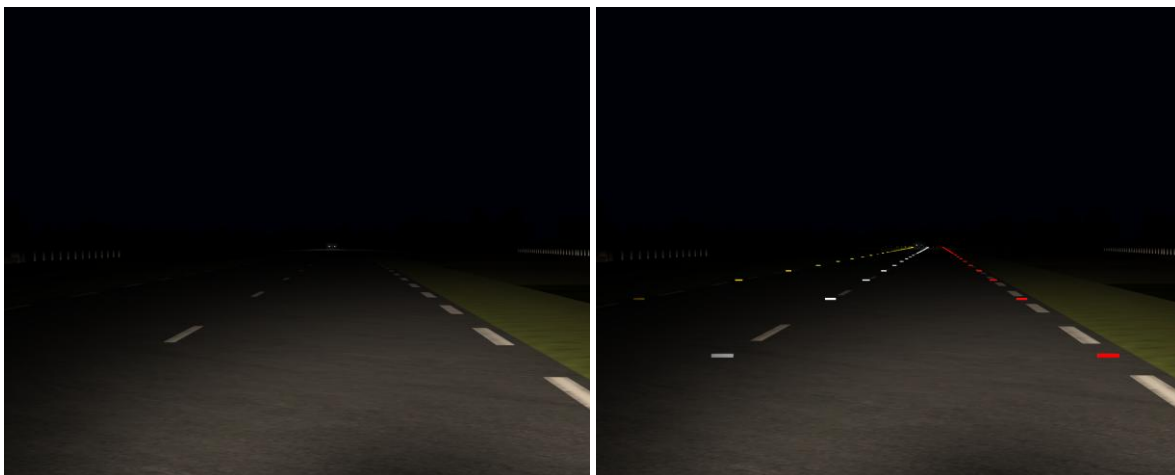
Figure 7. Oncoming vehicle on an unlit road and on a studded (nearside, central and offside) road.
