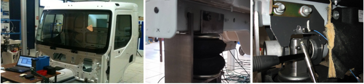
Figure 6: Test cabin measurements. Left: "body in white" test cabin; middle: truck frame link with the cabin suspension; right: impact hammer excitation.
