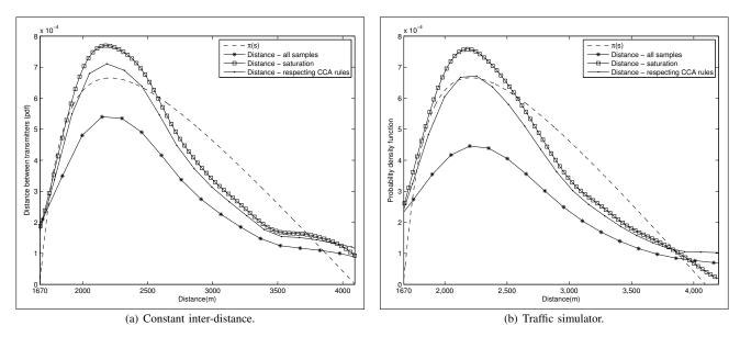
Fig. 13. No fading case: distribution of the distances between concurrent transmitters.
