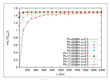
Fig. 3. Convergence of  $\frac{m(L)D}{L}$  as L increases for  $l(u) = P_t.min(c, \frac{c}{u^{\alpha}})$  and different value of  $\alpha$  and  $P_t$ . D is the solution of  $2l(\frac{D}{2}) = \theta$  with  $\theta = -99dBm$ .
