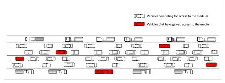
Fig. 1. Example of concurrent transmissions: the 802.11p MAC layer (CSMA/CA) set the rules to access the medium. Only red vehicles are allowed to transmit frames at the same time
