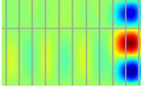
Figure 4: 11<sup>th</sup> mode of the ribbed plate with a frequency of 610.9 Hz presenting a localization of the vibration in the inter-ribbed spaces.
