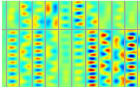
Figure 5: 288<sup>th</sup> mode of the ribbed plate with a frequency of 4190 Hz presenting complex vibratory phenomena.
