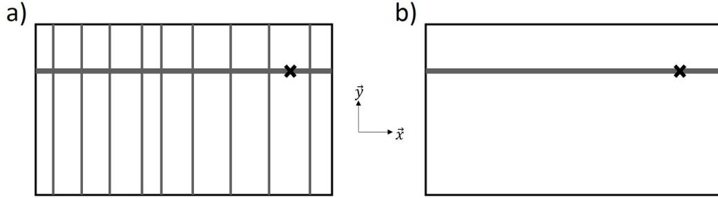
Figure 8: Drawing of two ribbed structures. (a) : simplified soundboard. ; (b) : soundboard without ribs.
