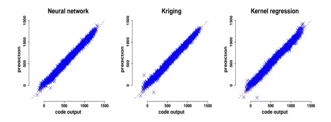
Figure 3: Plot of the metamodel predictions in the test base (y-axis), as a function of the Germinal output values (x-axis), for the neural networks (left), Kriging (middle) and kernel methods (right). Case of the original computations. The dashed lines is defined by y = x.
