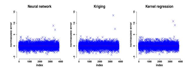
Figure 5: Plot of the normalized prediction errors (23) on the learning base (y-axis), as a function of the computation index (x-axis), for neural networks (left), Kriging (middle) and kernel methods (right). Case of the original computations. Two outliers stand out and correspond to the same computations for the three metamodels.
