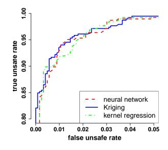
Figure 4: Plot of the "true unsafe rate" as a function of the "false unsafe rate", for varying values of the tuning parameter  $\tau$  in (22). The total number of unsafe  $\boldsymbol{x}$  is 385 and the total number of viable  $\boldsymbol{x}$  is 1228. The areas under the ROC curves are 0.9977 for Kriging, 0.9974 for the neural networks and 0.9972 for kernel methods.
