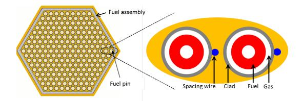
Figure 2: A schematic representation of a fuel pin and a fuel assembly in nuclear fast-neutron reactors.
