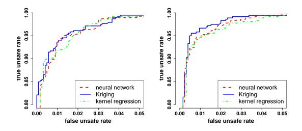
Figure 9: Plot of the "true unsafe rate" as a function of the "false unsafe rate", for varying values of the tuning parameter  $\tau$  in (22), for the original computations (left) and the updated computations (right). The total number of unsafe  $\boldsymbol{x}$  is 385 (left) and 359 (right), and the total number of viable  $\boldsymbol{x}$  is 1228 (left) and 1247 (right). For the updated computations, Kriging becomes more accurate than neural networks and kernel methods.
