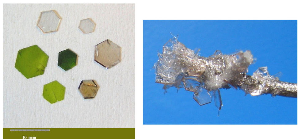
Fig. 4 \text{Fe}_x\text{Ga}_{1-x}\text{BO}_3 single crystals with different x (left) and \text{GaBO}_3 crystals on the seed holder (right)
