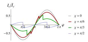
FIG. 2: Typical current-phase relations. The current is plot in units of  $\bar{I}_c = \gamma Ga(T)/(2e)$  for different magnetization angles  $\chi$  and b(T)/a(T) = 0.15, cf. Eq. (33). The critical current is achieved at phase  $\varphi = \pi/2$  for  $\chi = 0$  and  $\pi/6$ , and at phase  $\varphi = \pi - \chi$  for  $\chi = \pi/3$  and  $\pi/2$ .
