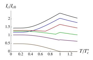
FIG. 5: Plot of the critical current  $I_c$  [in units of  $I_{c0} = \gamma G(\gamma_F h'/\gamma_S^2)^2/(2e)$ ] as a function of  $T/T_c^*$ , for  $h', T_c^* \ll \gamma_S$ , and different angles  $\chi = 0, \pi/6, \pi/4, \pi/3, 2\pi/5, \pi/2$  (from top to bottom).
