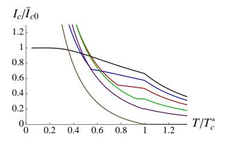
FIG. 6: Plot of the critical current  $I_c$  [in units of  $\bar{I}_{c0} = \gamma G[\gamma_F \gamma_S/(h'\Delta_0^*)]^2/(2e)$ ], with  $\Delta_0^* \approx 1.76T_c^*$ , as a function of  $T/T_c^*$ , for  $\gamma_F \ll \gamma_S, T_c^* \ll h'$ , and different angles  $\chi = 0, \pi/6, \pi/4, \pi/3, 2\pi/5, \pi/2$  (from top to bottom). Note that the critical current saturates at  $T \lesssim \gamma_F$  (not visible on the scale of the figure).
