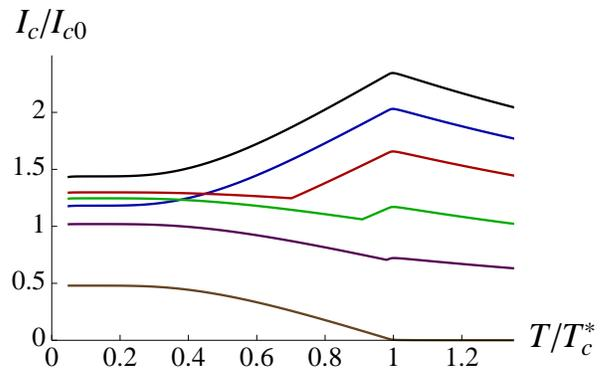
FIG. 5: Plot of the critical current  $I_c$  [in units of  $I_{c0} = \gamma G (\gamma_F h' / \gamma_S^2)^2 / (2e)$ ] as a function of  $T/T_c^*$ , for  $h', T_c^* \ll \gamma_S$ , and different angles  $\chi = 0, \pi/6, \pi/4, \pi/3, 2\pi/5, \pi/2$  (from top to bottom).
