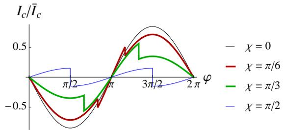
FIG. 2: Typical current-phase relations. The current is plot in units of  $\bar{I}_c = \gamma G a(T)/(2e)$  for different magnetization angles  $\chi$  and  $b(T)/a(T) = 0.15$ , cf. Eq. (33). The critical current is achieved at phase  $\varphi = \pi/2$  for  $\chi = 0$  and  $\pi/6$ , and at phase  $\varphi = \pi - \chi$  for  $\chi = \pi/3$  and  $\pi/2$ .
