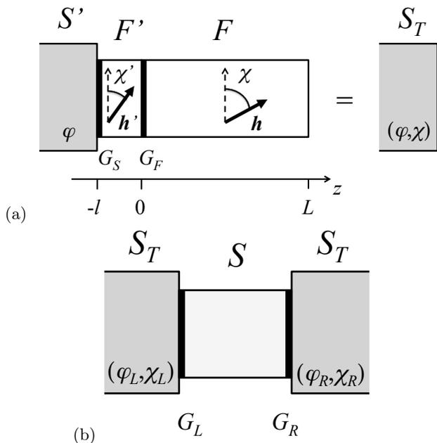
FIG. 1: (a) Realization of an effective triplet odd-frequency superconductor  $S_T$  by contacting a ferromagnetic  $F'/F$  bilayer with noncollinear magnetizations, with a relative angle  $\theta = \chi - \chi'$  between their directions, to a singlet even-frequency superconductor  $S'$ . (b) Effective  $S_T/S/S_T$  double Josephson junction formed with triplet odd-frequency superconducting leads connected through a singlet even-frequency superconducting layer.
