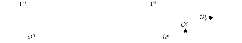
Figure 1: A 2D schematic view: unperturbed waveguide on left, perturbed waveguide (with two flies) on right.
