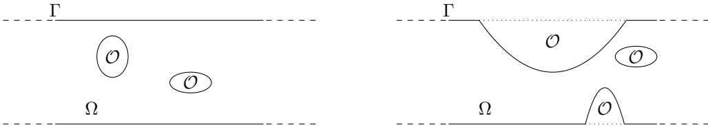
Figure 2: Examples of perturbed waveguides for which transmission invisibility cannot be imposed.
